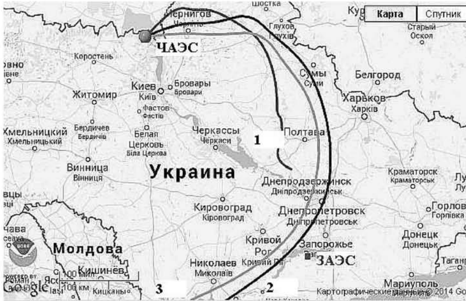
Fig. 4. Direct propagation path from the ChNPP (coordinates 51.39 N and 30.09 E) for 3 days (from 29.04.86 till 1.05.86, zero time), at heights of 20 m (line 1), 500 m (line 2) and 1000 m (line 3). At a level of 500 m, prevalence of pollution from Chornobyl is observed; the releases are directed toward S-E to the ZNPP, reaching the ZNPP location area at heights of 500 and 1000 m on 1 May
