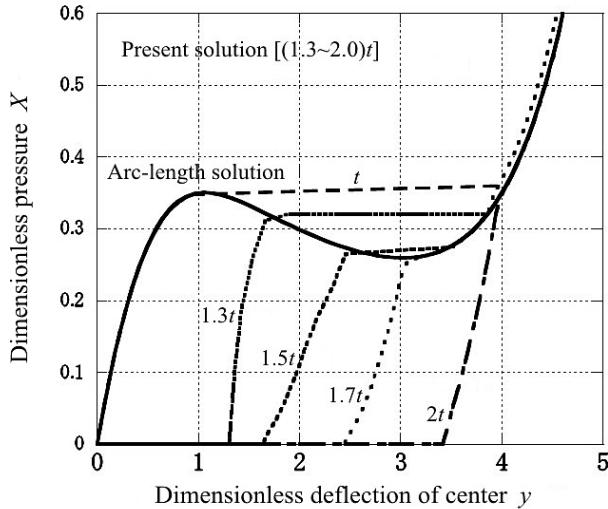
Fig. 7. Calculated critical snap-through arc-length solution results for  $\lambda = 3.8$  by present solutions ( $1.3t$ ,  $1.5t$ ,  $1.7t$ , and  $2t$ ), explicit solution ( $t$ ), and arc-length solution for clamped shallow spherical shells.
