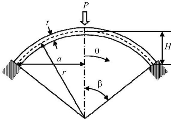
Fig. 1. Geometry of clamped shallow spherical shells.
