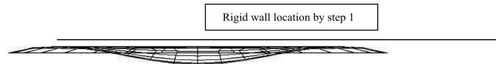
Fig. 8. Buckling shape of the top of a spherical shell by the procedure outlined in step 1 of the proposed method for the solution ( $2t$ ).
