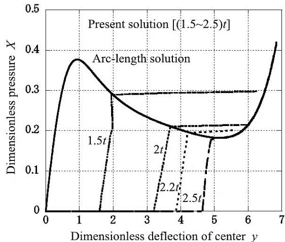
Fig. 9. Calculated critical snap-through arc-length solution results for  $\lambda = 4.6$  by the proposed procedure  $[(1.5\sim 2.5)t]$  and the arc-length solution for clamped shallow spherical shells.
