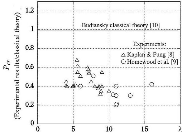
Fig. 2. Calculated solutions for classical theory and experimental results for clamped shallow spherical shells.
