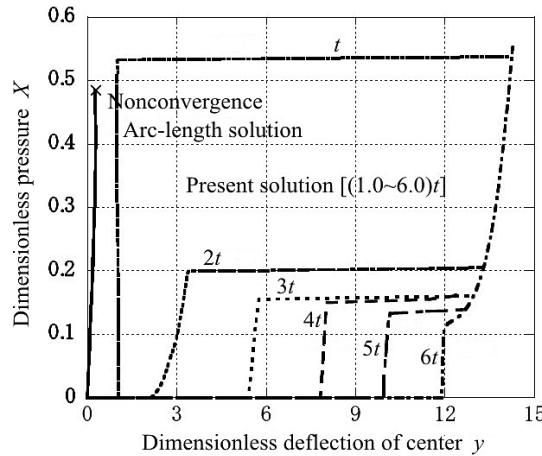
Fig. 10. Calculated critical snap-through arc-length solution results for  $\lambda = 6.5$  by the proposed procedure  $[(1.0\sim 6.0)t]$  and arc-length solutions (nonconvergence) for clamped shallow spherical shells.
