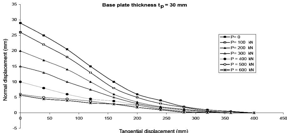
Fig. 16. Curves of the normal and tangential displacement of the 30 mm thickness base plate.
