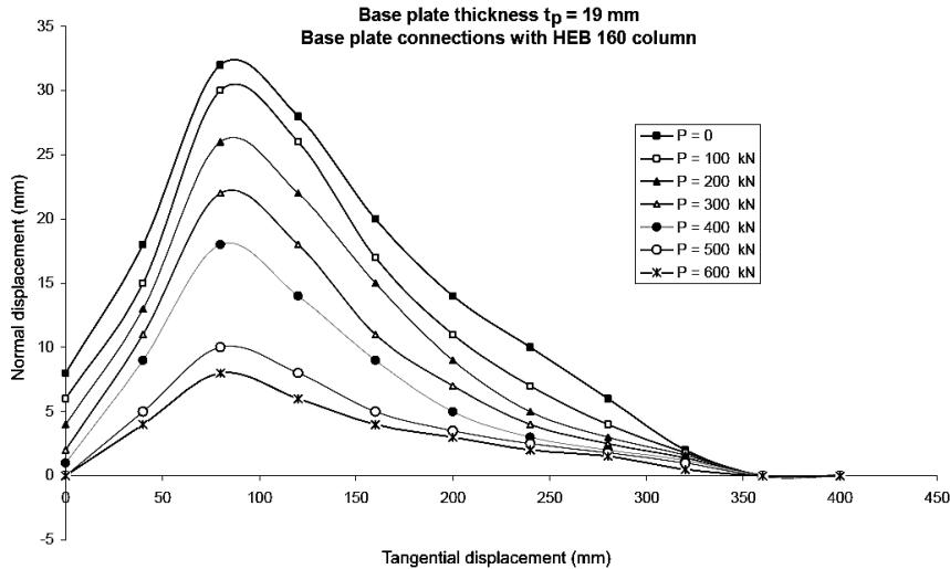
Fig. 15. Curves of the normal and tangential displacement of the 19 mm thickness base plate.
