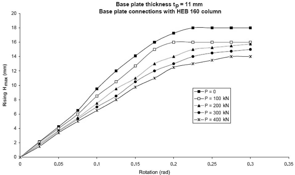
Fig. 10. Maximum rising-rotation diagrams for base plate thickness  $t_p = 11$  mm under various axial loadings. Base plate connections with HEB 160 column.
