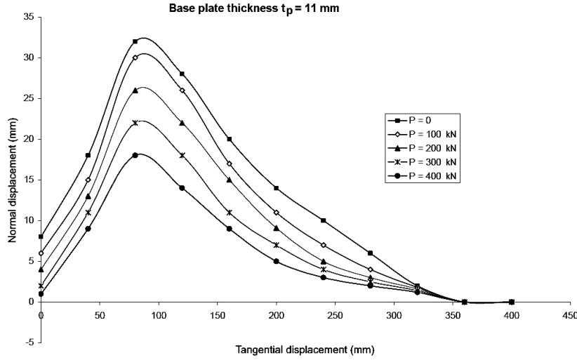
Fig. 14. Curves of the normal and tangential displacement of the 11 mm thickness base plate.
