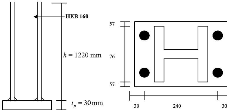
Fig. 6. Detail of four anchor bolts connection.
