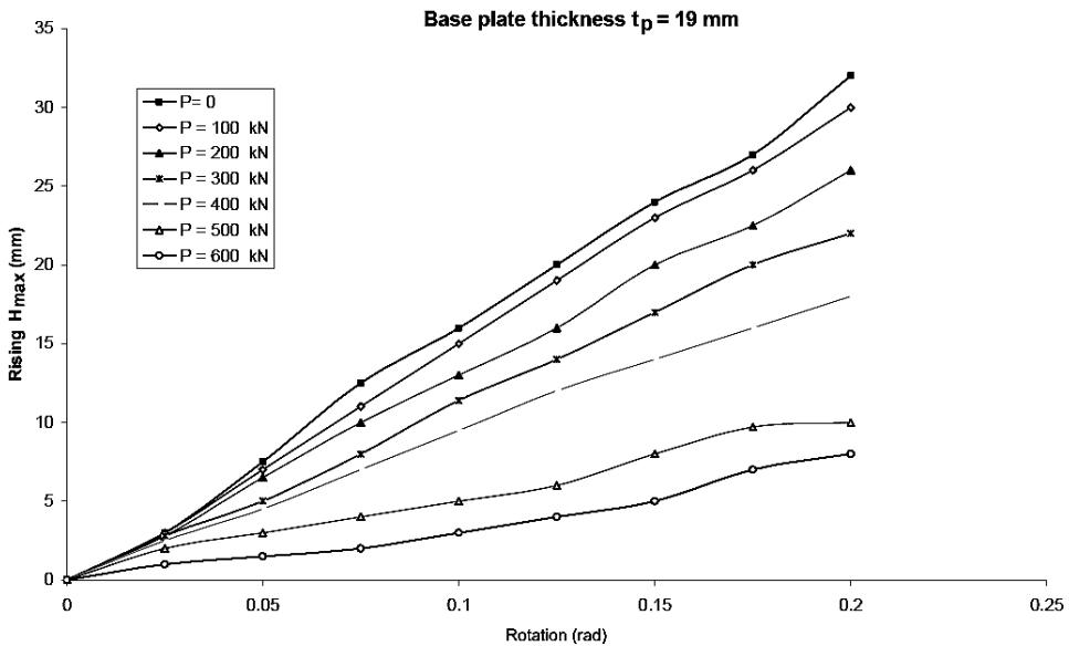
Fig. 11. Curves of the rising of the 19 mm thickness base plate under various axial loadings. Base plate connections with HEB 160 column.
