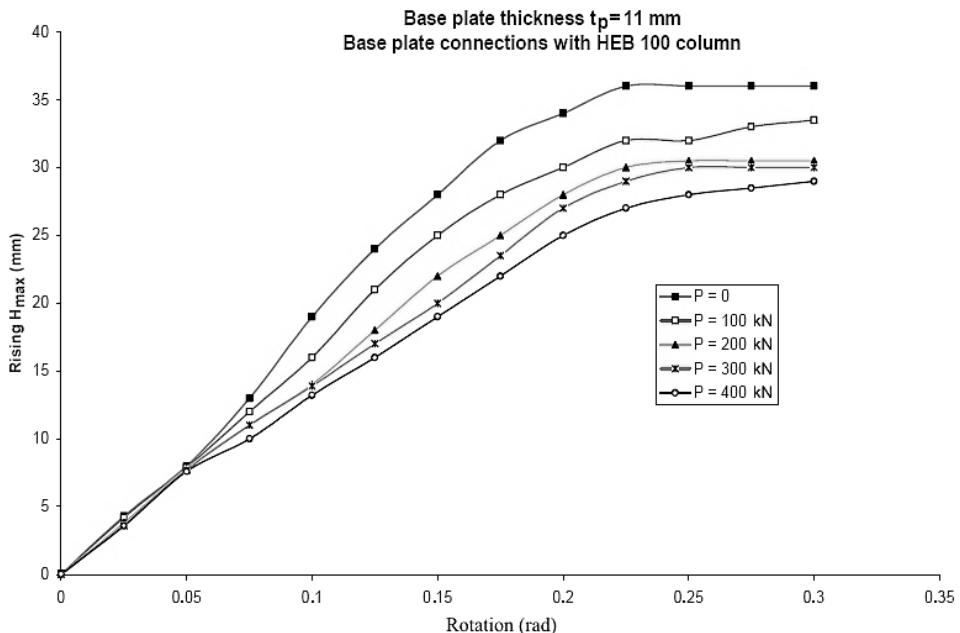
Fig. 9. Maximum rising–rotation diagrams for base plate thickness  $t_p = 11$  mm under various axial loadings. Base plate connections with HEB 100 column.
