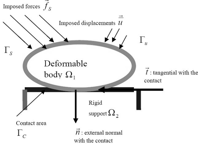
Fig. 1. Contact between a deformable body and a rigid body (the Signorini problem).
