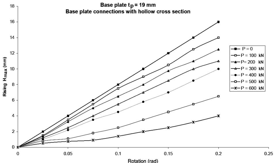
Fig. 13. Curves of the rising of the 19 mm thickness base plate under various axial loadings. Base plate connections with a hollow cross section.
