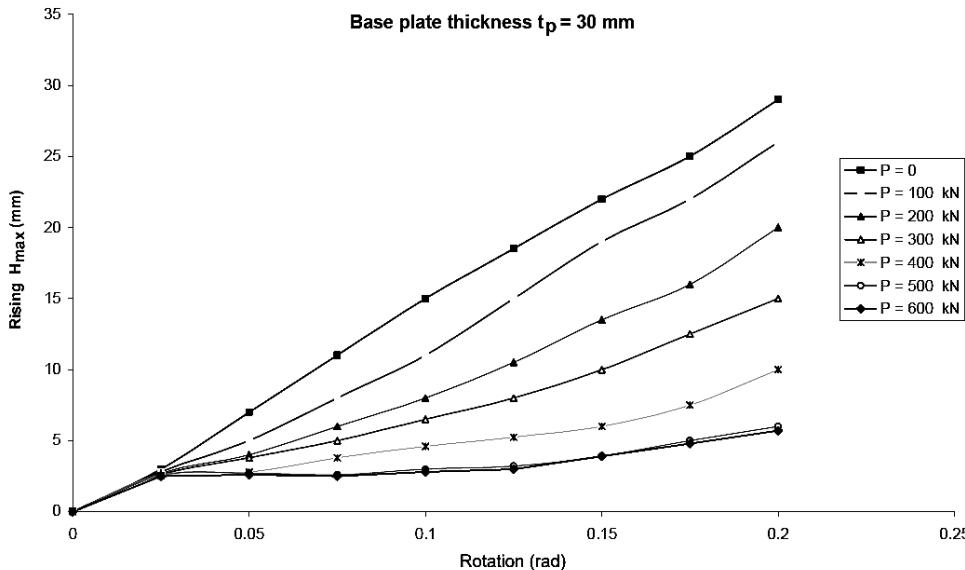
Fig. 12. Curves of the rising of the 30 mm thickness base plate under various axial loadings.
