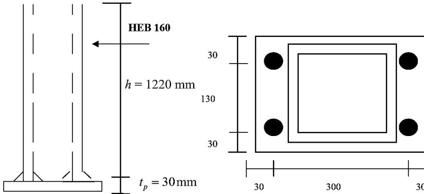
Fig. 7. Detail of four anchor bolts connection with a hollow cross section.
