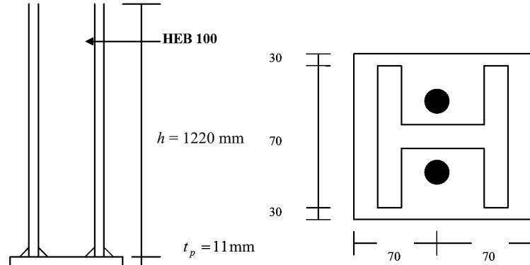
Fig. 5. Detail of two anchor bolts connection.
