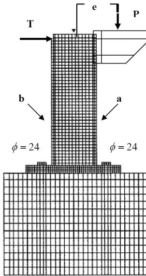
Fig. 8. Finite element mesh of the 3D model.
