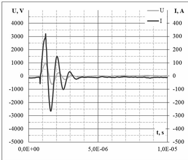
Fig. 2. Discharge current and voltage oscillogrames
