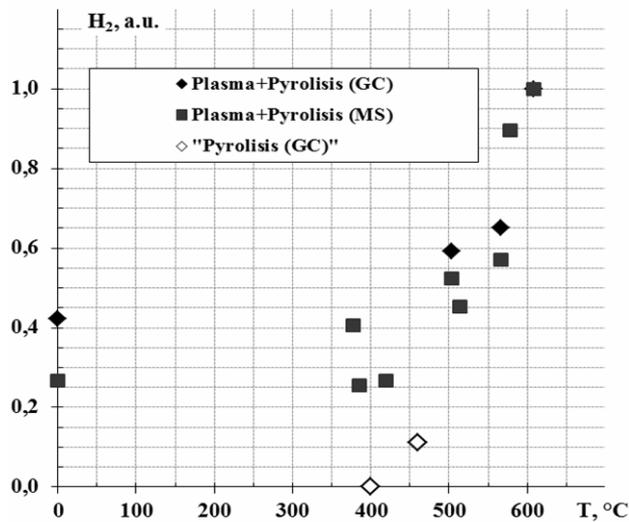
Fig. 3. H<sub>2</sub> intensity (MS) and partial H<sub>2</sub> content in syngas products (GC) after the ethanol reforming versus postdischarge pyrolytic chamber temperature
