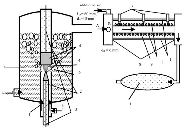
*Fig. 1. Schematic of ethanol pyrolysis after plasma-assisted reforming of ethanol in the DGCLW*
