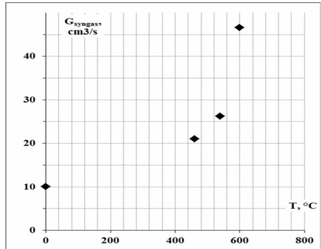
Fig. 5. The rate of syngas generation versus temperature in the pyrolytic chamber
