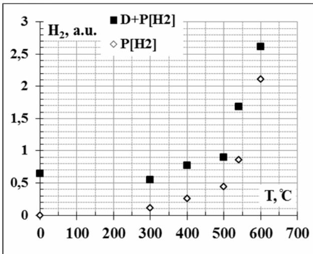
Fig. 7. H<sub>2</sub> intensity (MS) plasma reforming and partial oxidation pyrolysis versus pyrolytic chamber temperature
