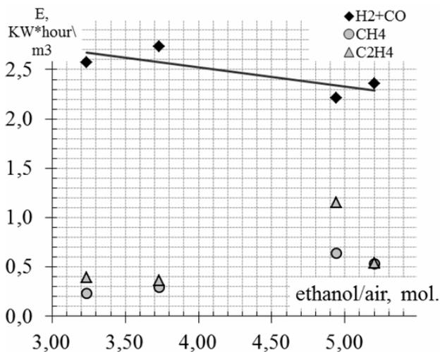
Fig. 6. Syngas components LHV versus ethanol/air molar rate
