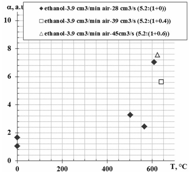
Fig. 4. Energy efficiency of ethanol reforming versus temperature in the postdischarge pyrolytic chamber
