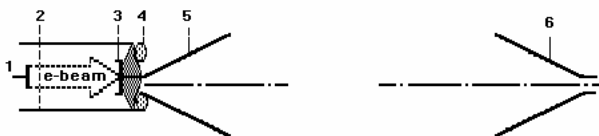
Fig. 1. Scheme of the experiments: 1 – cathode, 2 – e-beam, 3 – anode-collector, 4 – Rogovsky coil, 5, 6 – sending and pickup antennas
