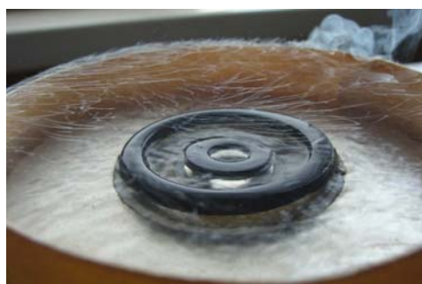
Fig. 2. Stable configuration of two levitating superconducting rings. Diameter of external ring is equal to 46 mm, diameter of internal ring - 19 mm
