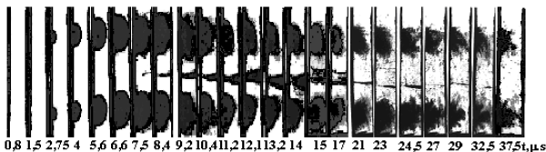
Fig.3. GPT spread from steel 12X18H10T (strip target)
