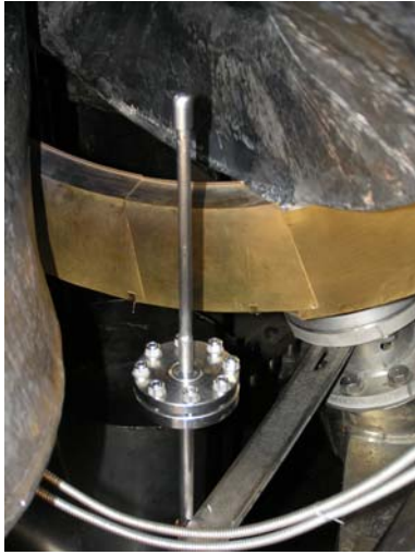
Fig.2. W-limiter diffusion membrane position in situ in U-3M vacuum chamber between two housings of helical windings of the toroidal magnetic field coils
