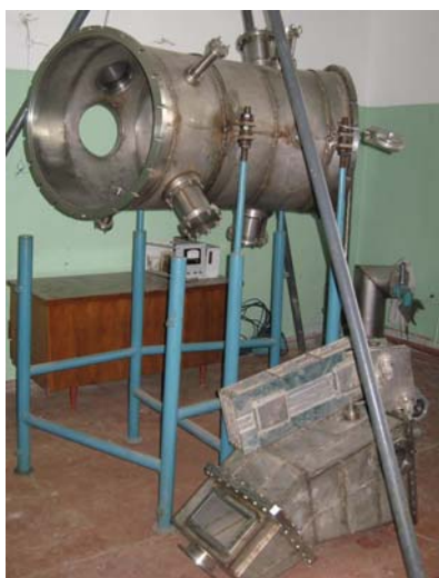
Fig. 8. Vacuum stand construction
