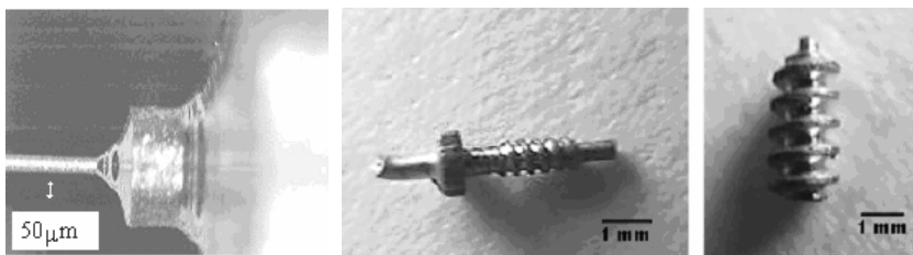
Fig. 2. Brass needle with diameter of 50 \mu m and examples of work pieces manufactured with the first micro machine tool prototype
