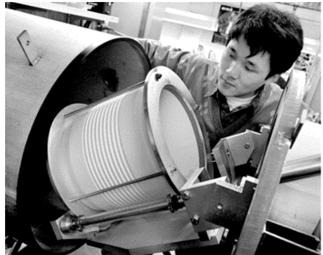
Fig. 5 Ceramic accelerator column in Mevva implanter
