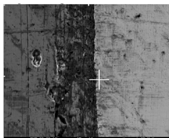
Fig.3. Metallographic section of a sample Cu -W after an irradiation by 40 pulses of plasma. The place of the local analysis of structure of W on the distance 2 microns from a surface is marked
