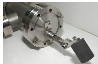
Fig. 4. Simple ion-pinhole camera fixed upon the manipulator prepared for COMPASS experiments
