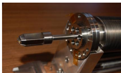
Fig. 2. Single-channel Cherenkov probe for ISTTOK
