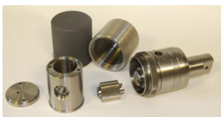
Fig. 5. Parts of the ion pinhole camera equipped with a rotated drum for several nuclear track detectors
