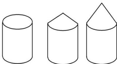
Fig. 1. Shapes of cathodes employed in this study
