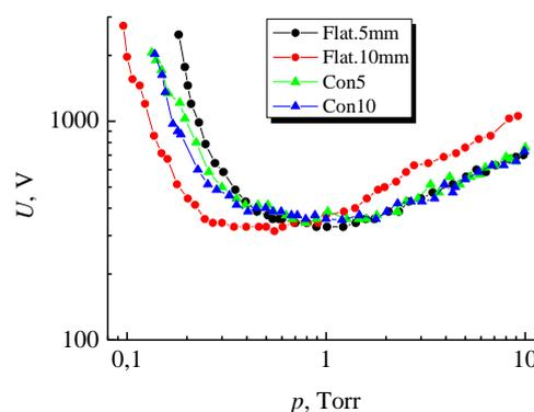
Fig. 3. Breakdown curves in nitrogen for the gap values between flat electrodes of 5 and 10 mm, as well as for conical cathodes
