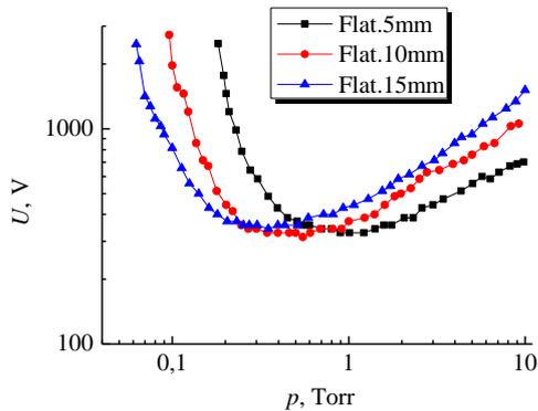
Fig. 2. Breakdown curves in nitrogen for the following gap values between flat electrodes: 5, 10, 15 mm
