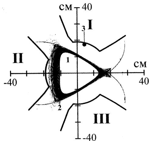
*Fig. 1. Cross section of the U – 3M magnetic configuration*
