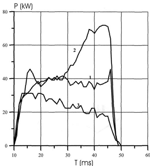
Fig 3. Temporal behaviour of radiative losses at three levels of RF power
