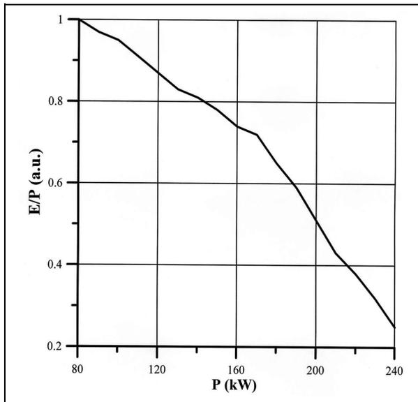
Fig 2. Normalize dependences radiative losses per pulse on the applied RF power
