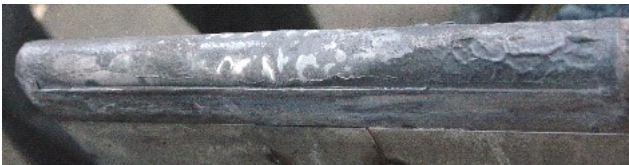
Fig.4. Li limiter surface after the exposition below the melting point
