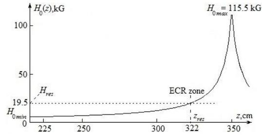
Fig. 2. On-axis distribution of the magnetic field strength  $H_0(z)$  in the GDT-like plasma
