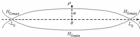
Fig. 1. Two-dimensional straight mirror-trapped magnetic field configuration
