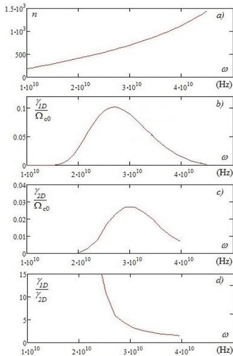
Fig. 3. The dispersion characteristics of ECWs versus  $\omega$  in a Gas-Dynamic Trap plasma
