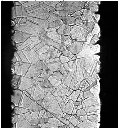
Alloy "A". #1 Irradiation dose is 5,066 eV per atom
