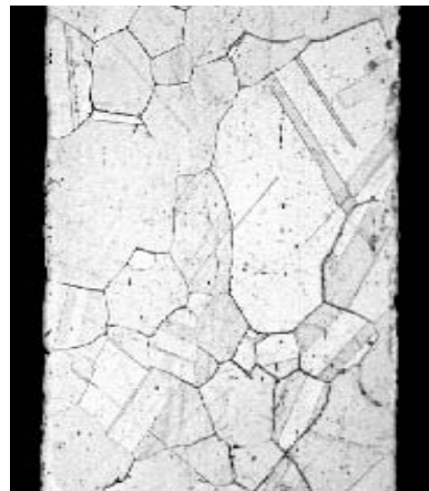
Alloy "B". #7 Irradiation dose is 64 eV per atom
