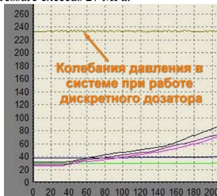
Fig. 9. Pressure fluctuations in the system when using discrete dispenser
