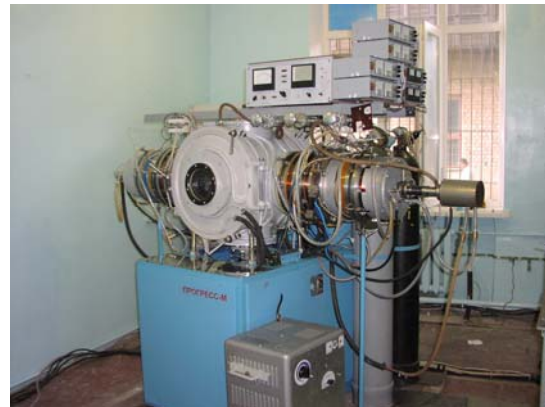
Fig. 2. Plasma coating setup with the vacuum arc source and MI filter
