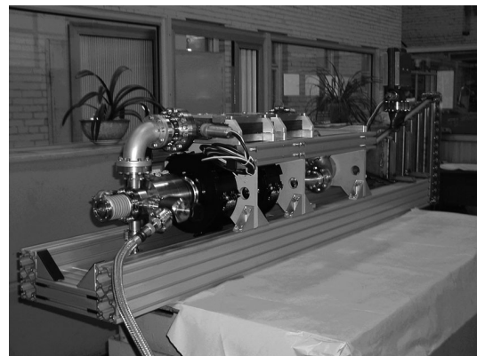
Fig. 7. Standing wave irradiator
