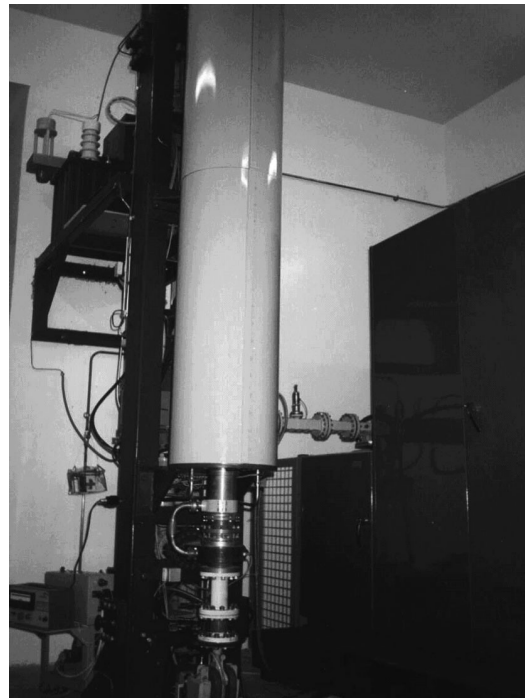
Fig. 4. Accelerator section and high-frequency generator
