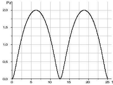
Fig.1. Dependence of longitudinal momentum of particle from its initial phase: 0, \pi/4, \pi/2, 3\pi/4, \pi at \mathbf{E} = 1
