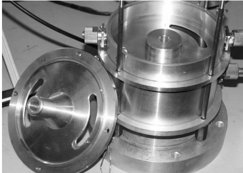
Fig.8: Accelerating structure (1:5 scale model)
