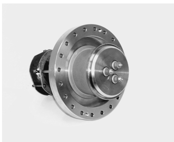
Fig. 2. Picture of ion source prototype (rear view).
