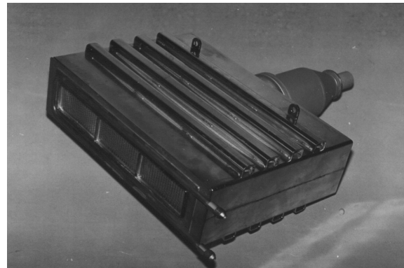
Fig. 5. Electron gun with a ribbon cathode.
