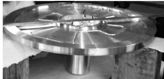
Fig. 2. Disk of accelerating structure during manufacturing
