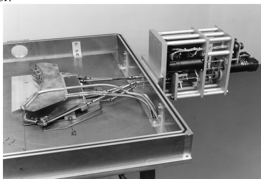
Fig.4. Test bench for the new deflector drive
