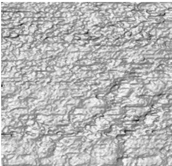
Fig. 6. The scanning tunnel microscopy of the center of Vanadium sample with thickness 0.29 mm. The irradiation of the sample was done by pulse of deuterium plasma at the distance 10 mm from anode of Plasma Focus. Size of the area 1.2 \times 1.2 \mu\text{m}
