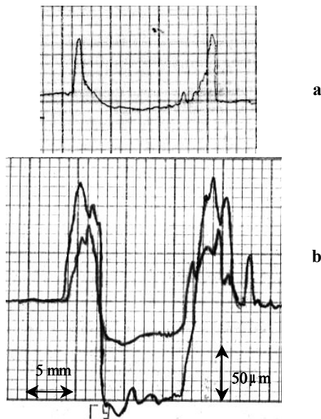
Fig. 3. Growth of erosion profile for Ti target under perpendicular plasma impact; a- 1 pulse, b- 5 and 20 pulses
