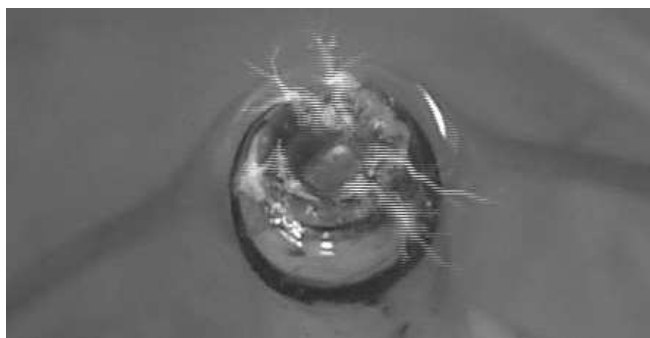
Fig. 3. Stationary discharge phase
