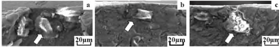
Fig. 3. SEM micrographs showing crack initiation site in laboratory air ( \sigma = 150 MPa): (a) AZ80, (b) AZ61, (c) AM60.
