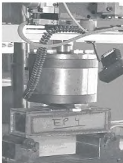
Fig. 4. Three-point bending test of welded box structures.
