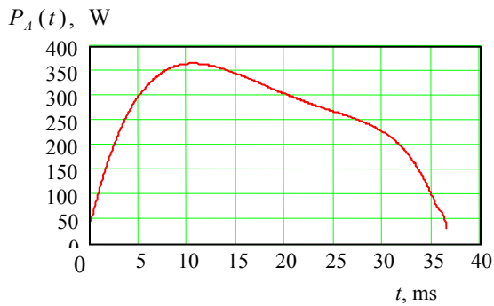
Fig. 5. Dynamics of arc power P_A(t) .
