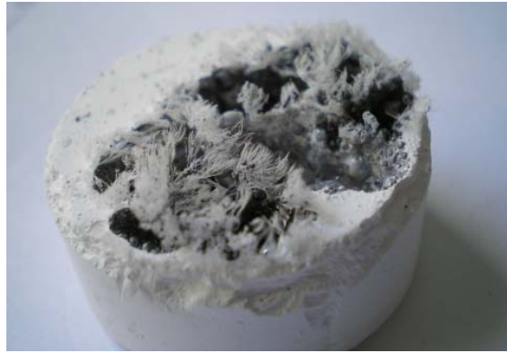
Fig. 2. Surface of compacted h-BN sample after heating in optical furnace.
