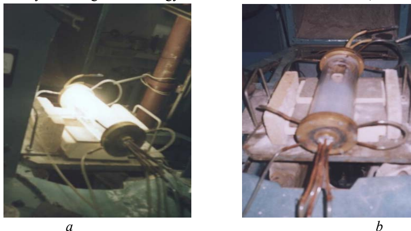
Fig. 1. Chamber for h-B transformations: a — during the heating; b — after experiment.
