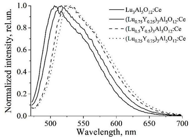
Comparison of the normalized luminescence spectra of composite scintillators based on grains  $(Lu_xY_{1-x})_3Al_5O_{12}:Ce$  (grains size 0.3...0.5 nm) with excitation of the light wavelength of 460 nm
