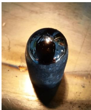
Fig. 8. Photo of the working material, molybdenum, after its use in the main arc discharge
