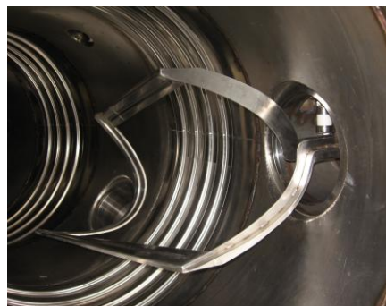
Fig. 2. The frame antenna inside U-2M chamber
