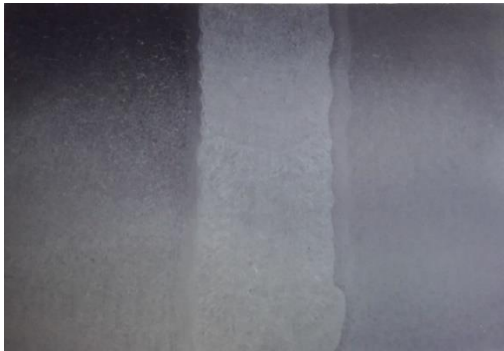
Fig. 2. Microstructure of the metal of the welded joint of the rotor made of steel 25H2NMFA. \times 11
