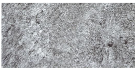
Fig. 1. The structure of the base metal of welded joints of steel 25H2NMFA. \times 400
