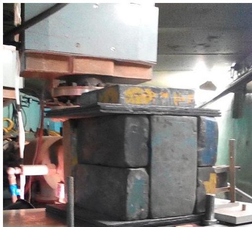
Fig. 3. Photo of a reflector with lead shielding on the axis of the LUE-30 accelerator
