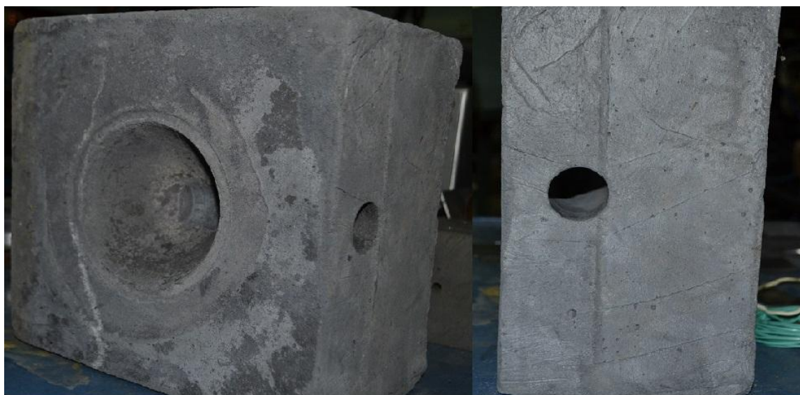
Fig. 2. Photo of a reflector made from a cement-graphite mixture with a working area in the form of a hemisphere. On the left is a view of the working area, on the right is a hole for passing the beam
