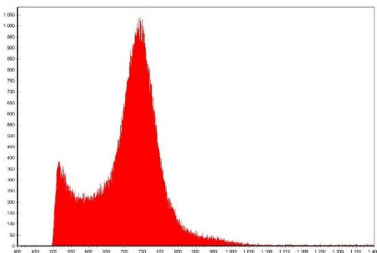
Fig. 5. One transistor at the input of the CSA. Energy resolution 8.36 keV
