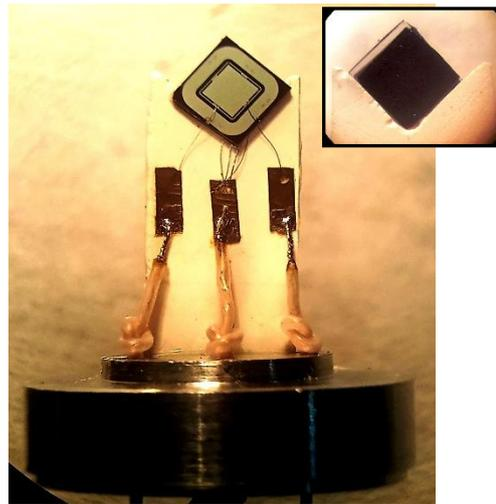
Fig. 3. Detecting module 2×2 mm with a converter and an absorbing gasket, in the upper right corner – a view of the detector from the back side
