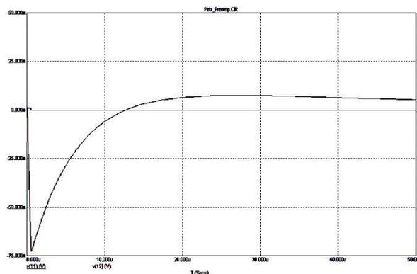
Fig. 8. The shape of the pulse at the output of the CSA obtained during the simulation
