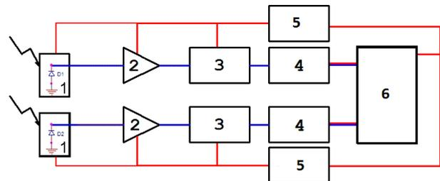
Fig. 4. Block diagram of a two-channel spectrometric system [8]: 1 – detecting modules; 2 – charge-sensitive amplifiers; 3 – spectrometric amplifiers;
