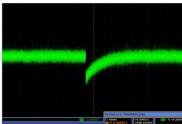
Fig. 9. A typical oscillogram of the pulse at the output of the CSA
