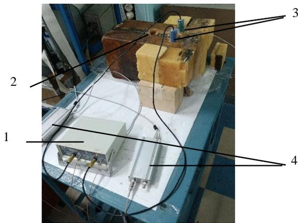
Fig. 10. Two-channel spectrometric system for registering the energy levels of conversion electrons: 1 – main block of the spectrometric system; 2 – neutron source IBN-21 in the middle of the paraffin block; 3 – detector modules with remote preamplifiers; 4 – ADC of the first and second channels
