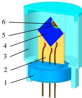
Fig. 2. Detecting module with converter and absorbing gasket: 1 – base; 2 – detector holder; 3 – housing;
