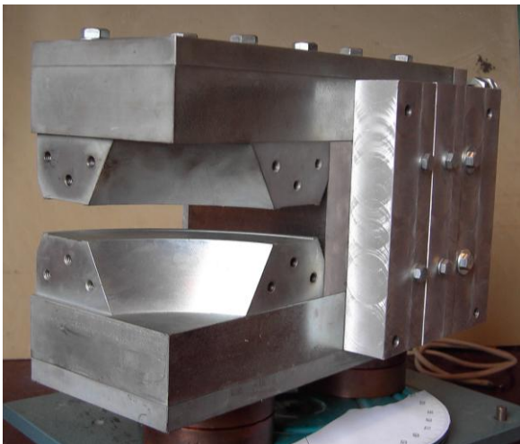
Fig. 7. General view of Nd-Fe-B magnetic system of 23 MeV electron accelerator
