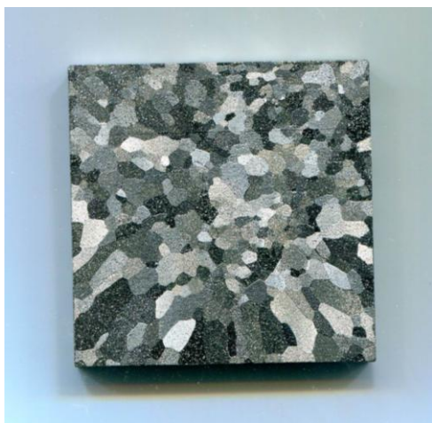
Fig. 3. Vacuum melted plate W 48 \times 48 \times 4.7 mm with Ta coating 250 \mu\text{m} thick. The grain structure of the substrate is developed in the coating due to epitaxial growth
