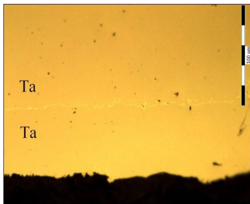
Fig. 5. Ta coating (bottom) on a Ta substrate. Coating temperature 1600; application time 90 min; thickness 65...75 μm; microhardness of the substrate 2.04 GPa; coatings – 2.26 GPa
