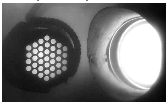
Fig. 2. Photo of the ICP source and magnetron discharge in simultaneous operation in Setup 1
