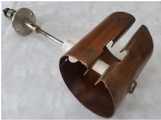
Fig. 1. Resonant frequency tuner of the type of the loop with the concentrated capacity
