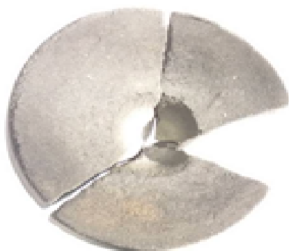
Fig. 4. Cracks at the ends of the container
