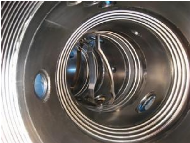
Fig. 1. THT antenna was made from crankshaft one by replacing central crankshaft strap with the straight one
