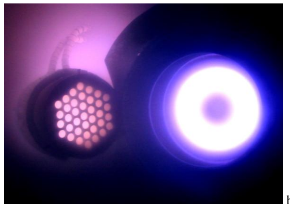
Fig. 1. Scheme of the experimental setup (1 – substrate holder, 2 – magnetron, 3 – RF ICP source) (a); Photo of the ICP source and magnetron discharge in simultaneous operation (b)
