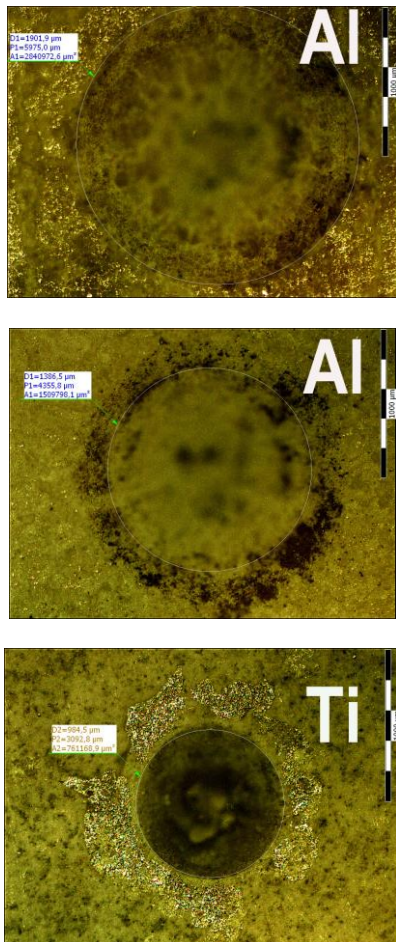
Fig. 10. Indenter traces on adhesion-tested specimens
