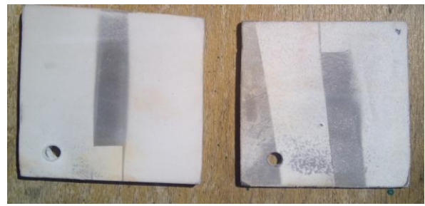
Fig. 12. The tested specimens made of Al and Ti with platinum strips
