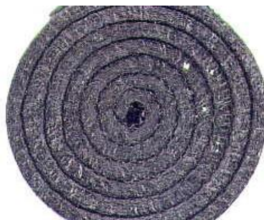
Fig. 4. External view of the layered C-C- composite after oxidation at 900°C in the muffle furnace
