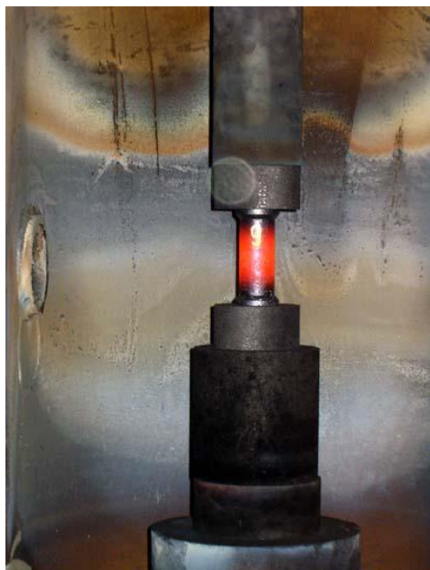
Fig. 6. Photo of the experiment on the investigation into the erosion of C-C composite resistance in the air
