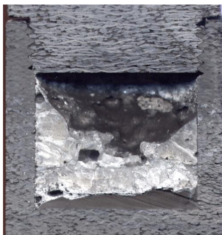
Fig. 3. Section of the container with a frozen melted salt after 20 “heating-cooling” cycles
