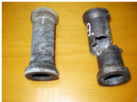
Fig. 7. Appearance of the samples after corrosion tests in the air
