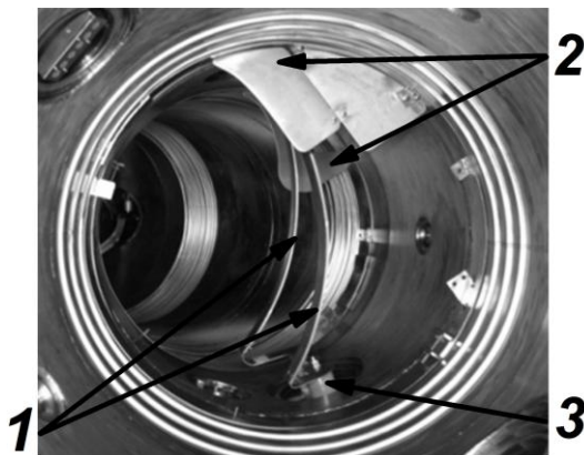
Fig. 3. Photo of the antenna inside the U-2M device: 1 – straps; 2 – limiters from both sides of antenna; 3 – fluoroplastic isolator covered with a quartz tube
